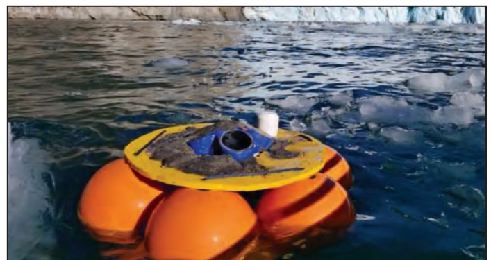
Sentinel V ADCP during recovery after being deployed for two weeks near LeConte Glacier.
